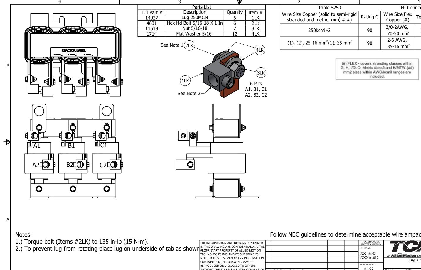
**IHI Connectors** Torque (All Drive Means) 375 in-lb (42.4 N-m) 275 in-lb (31.1 N-m)
