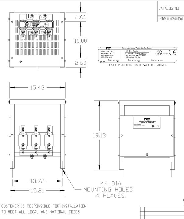
NEC NEC MOTOR MOTOR WATTS VOLTAGE APPROX. WEIGHT-LBS TORQUE (LB-IN) HP CURRENT  $\Box \Box \Box \Box \Box$ KDRULH24HE01 208/240 275 60 169 220 81
