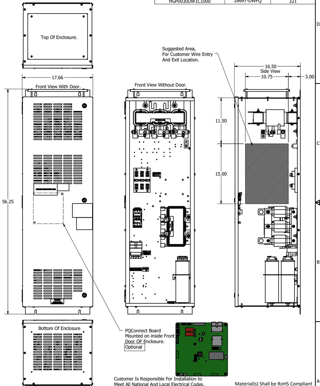
Note: Customer is responsible for proper cooling of filter components on open panels. Capacitors Maximum Ambient 50°C
