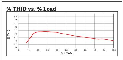
At standard test conditions of 1.5% source impedance and a VFD with 3% line reactance at full load, the HGP with PQconnect will provide 5% or lower THID at 50% of load.
