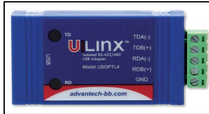
Figure 73: B&B SmartWorx, Inc Model: USPTL4 model RS-422/485 converter
