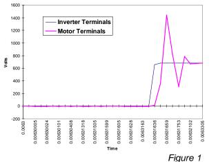
Also, recall that these voltage spikes can have a rise time, dV/dT, in excess of 7500 V/\subseteqs. This can have an extremely detrimental effect on the motor windings and on the insulation system, often causing premature motor failure. Most motor manufacturers believe that the life of the motor will be greatly extended by limiting both the magnitude of the voltage spikes to levels below 1000V and the dV/dT at the motor terminals to levels less than 1000 V/\subseteqs.
